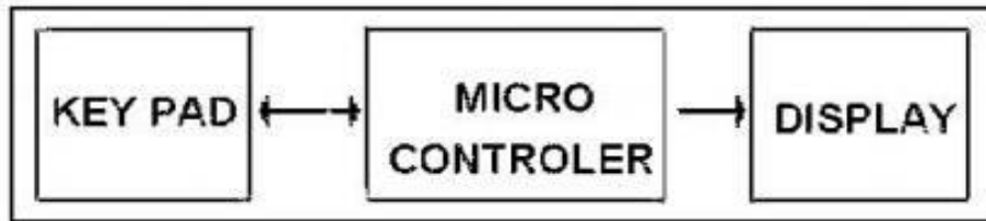
Fig 5.2 Interfacing Keyboard to 8051 Microcontroller
