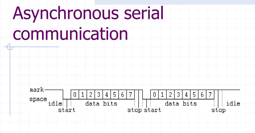
In this diagram, two bytes are sent, each consisting of a start bit, followed by eight data bits (bits 0-7), and one stop bit, for a 10-bit character frame.
