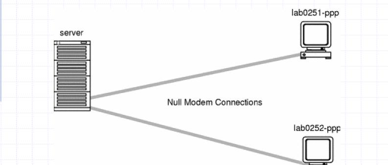
In this example, the server has two asynchronous null modem connections to the clients lab0251-ppp and lab0252-ppp. The modem keyword in the link.conf file is always set to none, and a dummy telephone number is assigned to the server.
