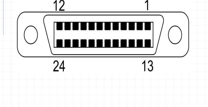
DIO1 Data input/output bit. Pin 1 Data input/output bit. Pin 2 DIO2 DIO3 Data input/output bit. Pin 3 DIO4 Data input/output bit. Pin 4 Pin 5 EOI End-or-identify. Pin 6 DAV Data valid. Pin 7 NRFD Not ready for data. NDAC Not data accepted. Pin 8 IFC Interface clear. Pin 9 SRQ Pin 10 Service request. ATN Pin 11 Attention. Pin 12 SHIELD
