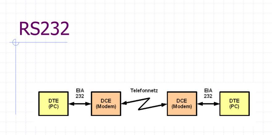
Data circuit-terminating equipment (DCE) and data terminal equipment (DTE) network. Telefonnetz refers to a telephone network; EIA-232 is an old name for RS-232, the serial communication standard.
